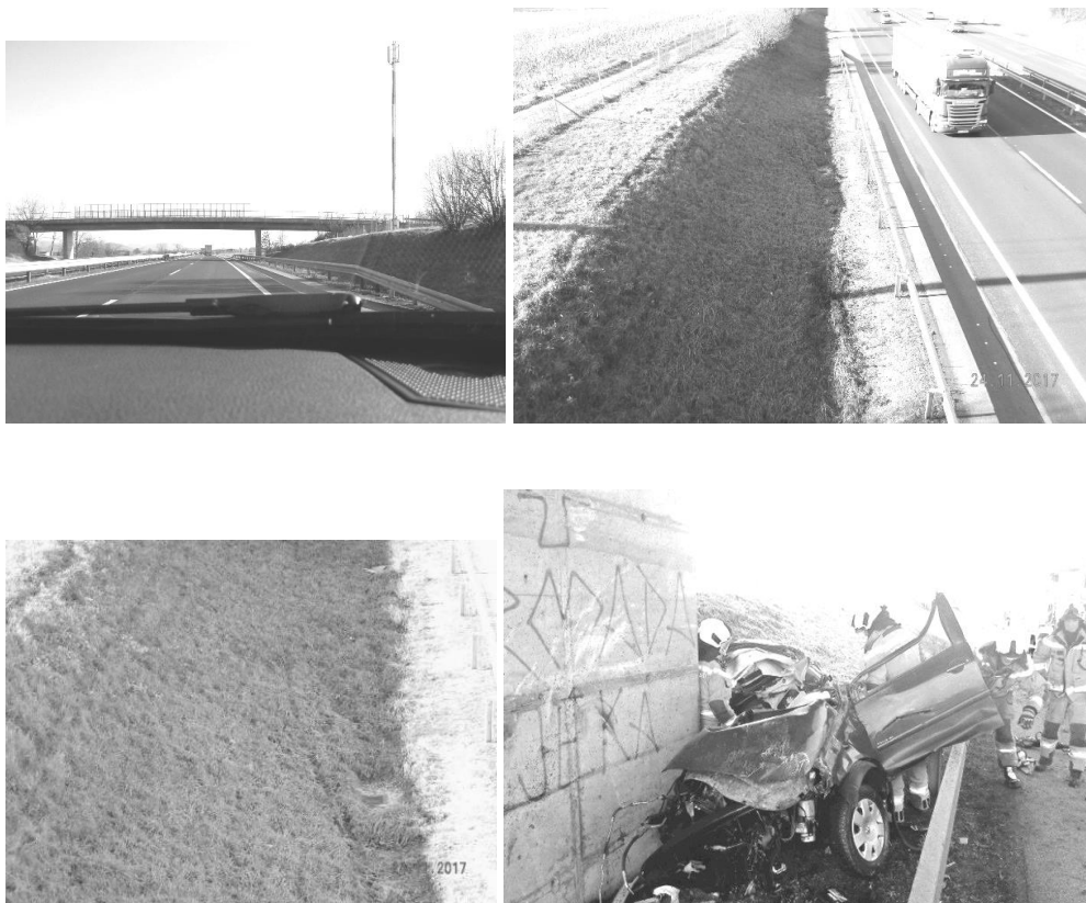
Figure 7: Tracks show that the car had been catapulted on inclined end terminal thrown on entrenchment and sliding along a trench finished in the pillar of an overpass.
