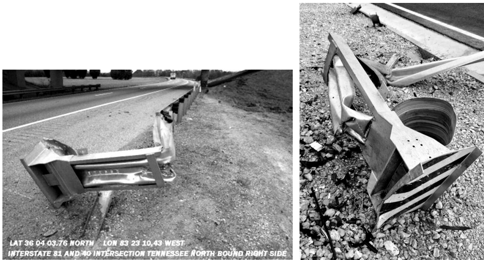
Figure 5: Terminal that fail to function properly in 2012 and the same type of terminal in our region in 2022(on the right). Same type malfunction.
